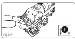
Re-attach nozzle guard by aligning the four (4) tabs in the base slots. Rotate nozzle guard back in place (Fig. 6/7).
